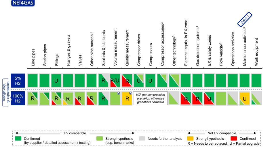
1. Thermowells, cleaning chambers, isolation couplings 2. Fuel path incl. regulation station, anti-surge system 3. Filters, coolers (only on CS), CP, TDW, TZB 4. Incl. EPS 5. Incl. vibrations and pulsations 6. Cleaning & inspection, venting and other manipulations, excavations
